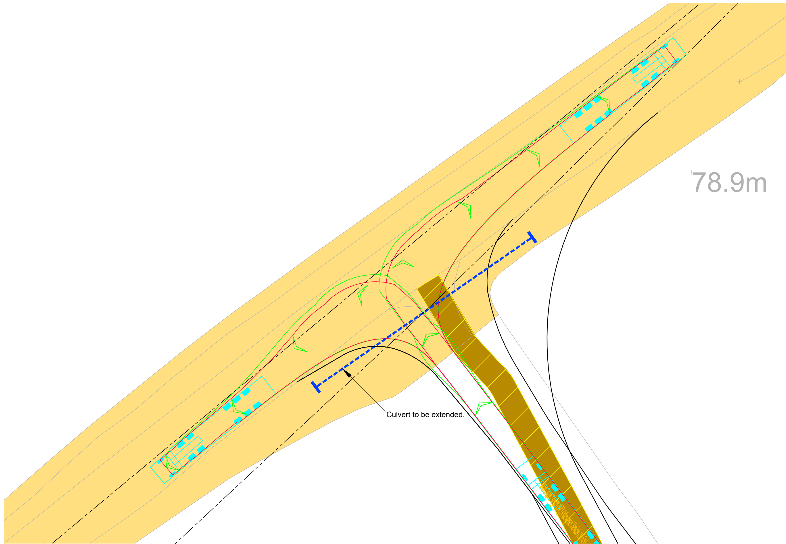
Swept Path Analysis of a 16.5m HGV Exited Scale 1:250
